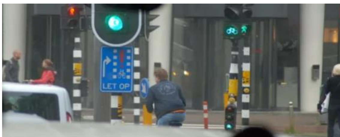
Figure 2.5.6 Example from the Netherlands of traffic signals + give way signage controlling turning traffic and cyclists
