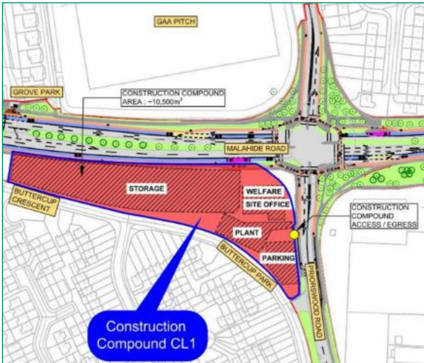
Figure 2.4.7: Extract of Image 5.1 of EIAR Chapter 5 Construction
